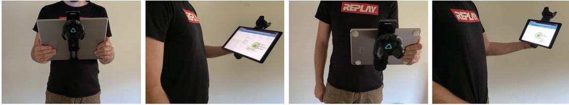
**Figure 4.1:** Vive tracker attached to tablet device with tripod mount. On the two pictures on the left, attached to the iPad Pro at backside and on top edge respectively, on the two pictures on the right on the iPad Air
