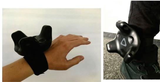
**Figure 2.14:** Vive trackers attached to wrist and ankle to track leg and arm movements for animating the prototype's player avatar (Caserman et al., 2019)
